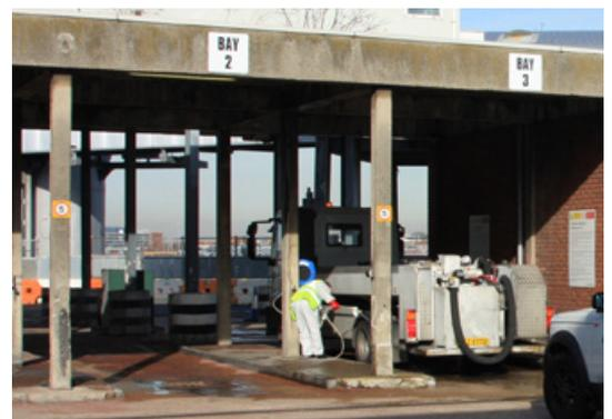
One of Heathrow's aircraft wastewater vehicles, transporting sludge to the Central Area Sanitation unit.
